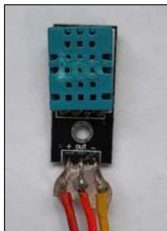
Fig.2 DHT11 Temperature and Humidity Sensor
