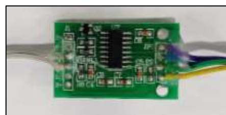
fig.8 24-bit analog to digital converter
